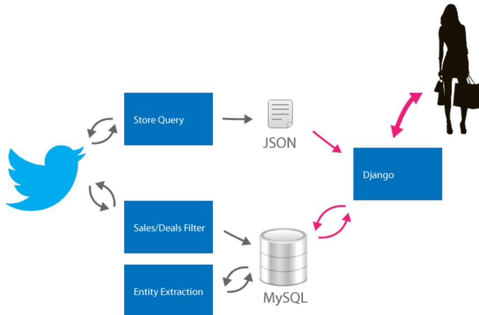
The figure above shows an overview of the SaleCloud architecture beginning (on the left) with retrieving sales and deals related tweets from Twitter and ending (on the right) with a UI that is delivered to the user via the Django web framework. The backend architecture is divided into two main parts: (1) the Store Map Section, and (2) the Entities Section.
