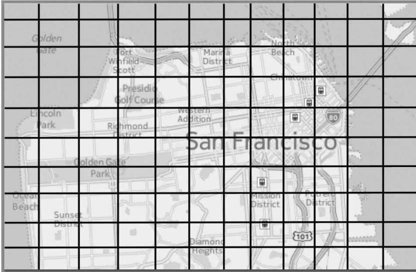
Once the image is divided into smaller squares (constructor is set), the algorithm accepts x,y coordinates of the points to be plotted. It then checks which square the x,y point plots to. Once identified, it returns the midpoint of that square. Thus, in this manner, if we have 2 or more tweets falling within a smaller square, they both would point to the same coordinates
